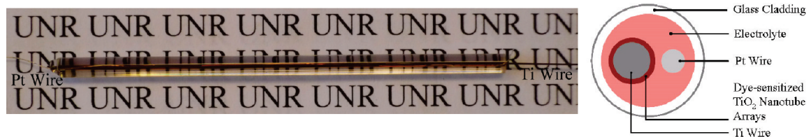
Scheme 1. Digital Photograph of a Prototype DSPVW and Its Schematic Cross Section
